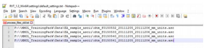
6. To batch process simple double click open the RVT tool and Click to Continue button and the tool will run without the GUI.
